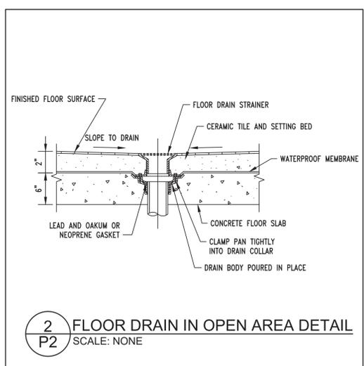
**2** FLOOR DRAIN IN OPEN AREA DETAIL
